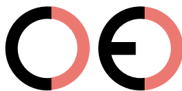
False CE Mark (too far)
